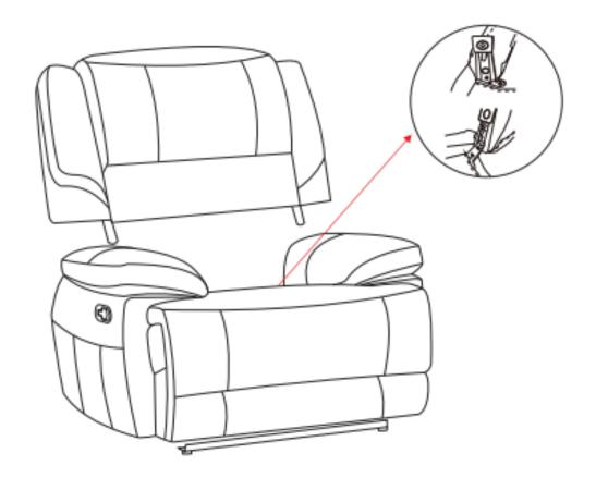
Note: To remove backrest, carefully lift tab using flat head screwdriver and slide backrest away from seat.
